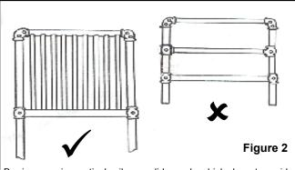
Barriers require vertical rails or solid panels which do not provide footholds or present entrapment hazards.
